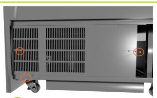
Remove the screws that hold the rear grill on to the rear of the cabinet and move the grill out of the way
