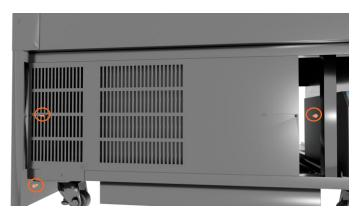
Place the rear grill back into position and reinstall the screws
