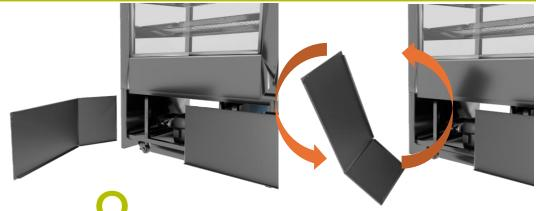
Slide the side piece of the baffle out and rotate it as shown
