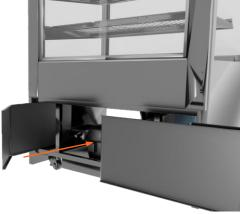
Slide the side piece of the baffle back into the cabinet, hard against the inner wall of the cabinet
