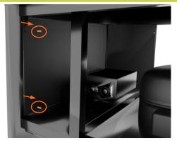
Remove the 2 screws holding the side piece of the baffle to the cabinet at the rear of the cabinet
