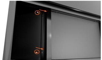
Reinstall the screws that attach both baffle pieces together
