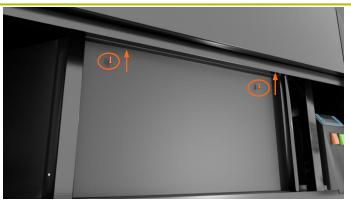
Attach the front/rear piece of the baffle to the cabinet by inserting the two screws upwards through the attachment holes
