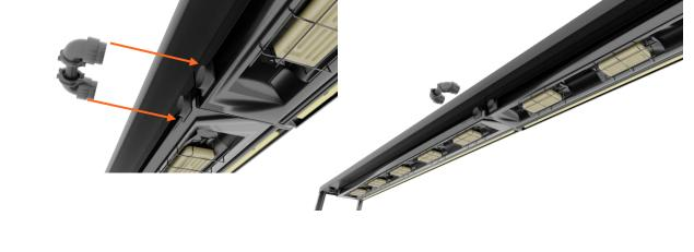
Once the heat bars have been installed into the pass-through end-to-end, a connecting cable can be plugged into the end sockets of each heat bar. Doing this allows up to 3 heat bars to run in series off one larger electrical box, one controller and one power cable.
